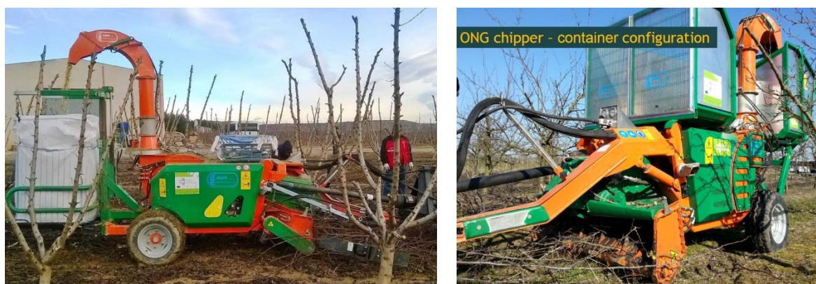
Figure 11. ONG PC50 chipper, in big bag and in container configuration (Pari, 2015).
