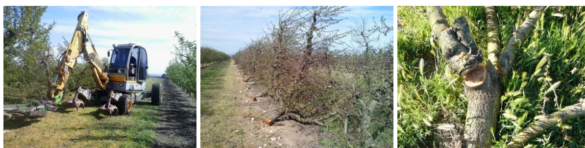
Figure 13. Walking excavator with shear for tree cutting; peach tree field after tree cutting; detail of tree preparation prior feeding into the chipper.
