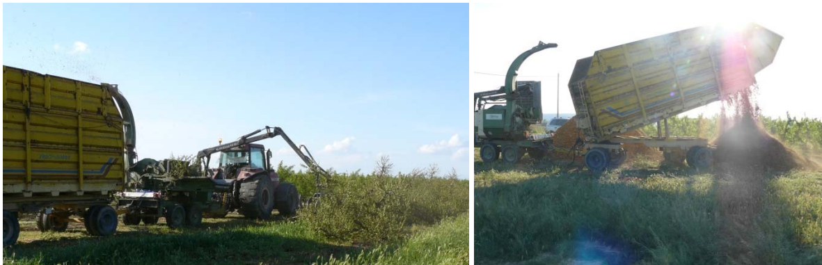
Figure 14. Forestry chipper fed with bundles of fruit tree stems and branches; downloading of the chips in provisional yard at roadside.
