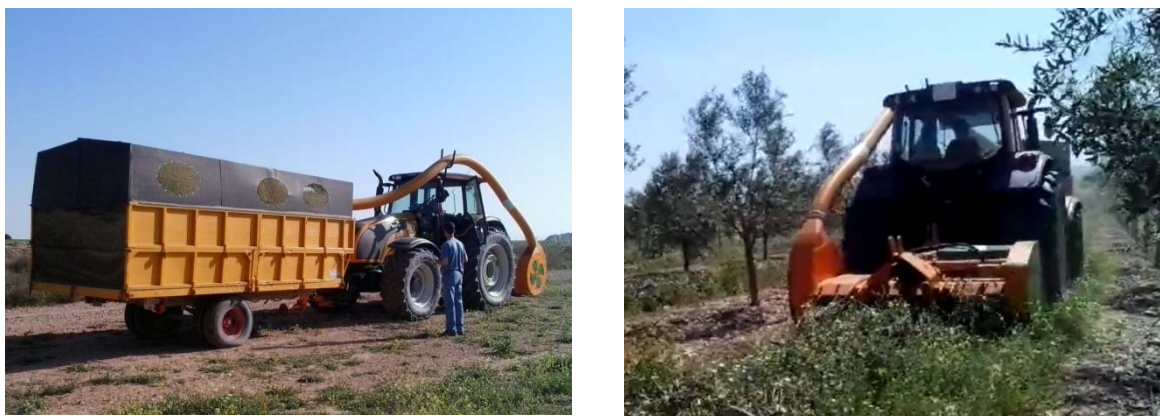
Figure 12. ONG PC50 chipper, in big bag and in container configuration (Pari, 2015).
