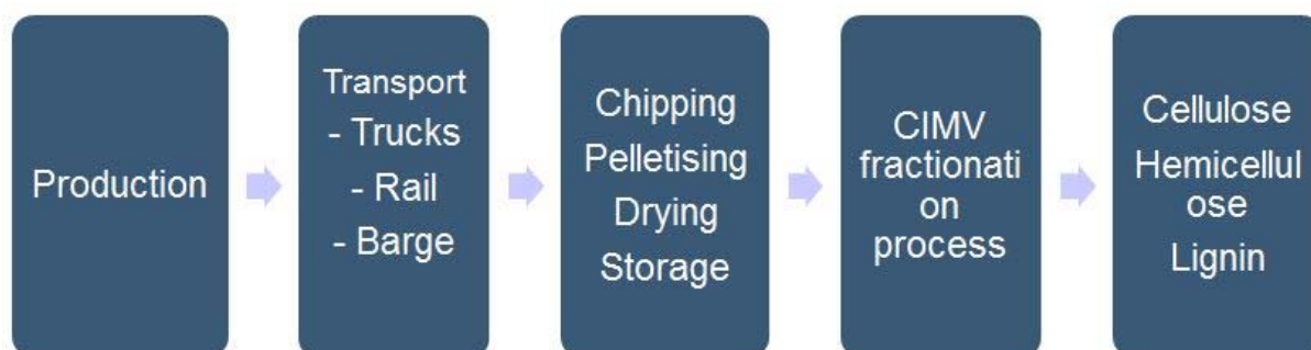
Figure 6. Schematic representation of the biomass value chain in the Biocore project (Biocore, 2014).
