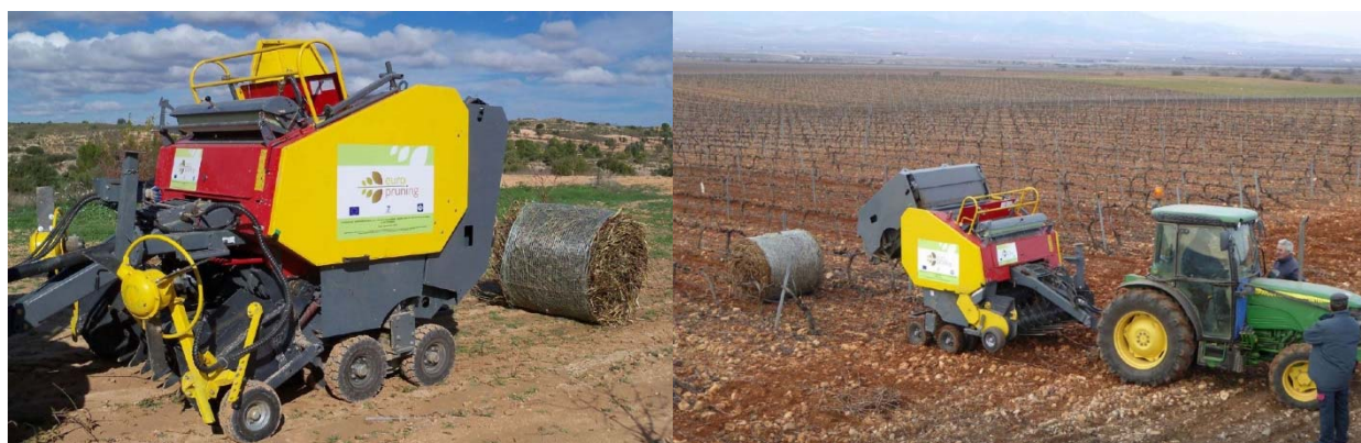
Figure 10. Pruning round baler during the performance tests on almond orchard in Alcaniz, Spain and in the pilot experience with vineyard in Carineña, Spain (Pari, 2015).
