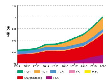
PUR: Polyurethane, PET: Polyethylene terephthalate, PBAT: Polybutyrate, PA: Polyamide, PHA: Polyhydroxyalkanoate, PLA: Polylactic acid
