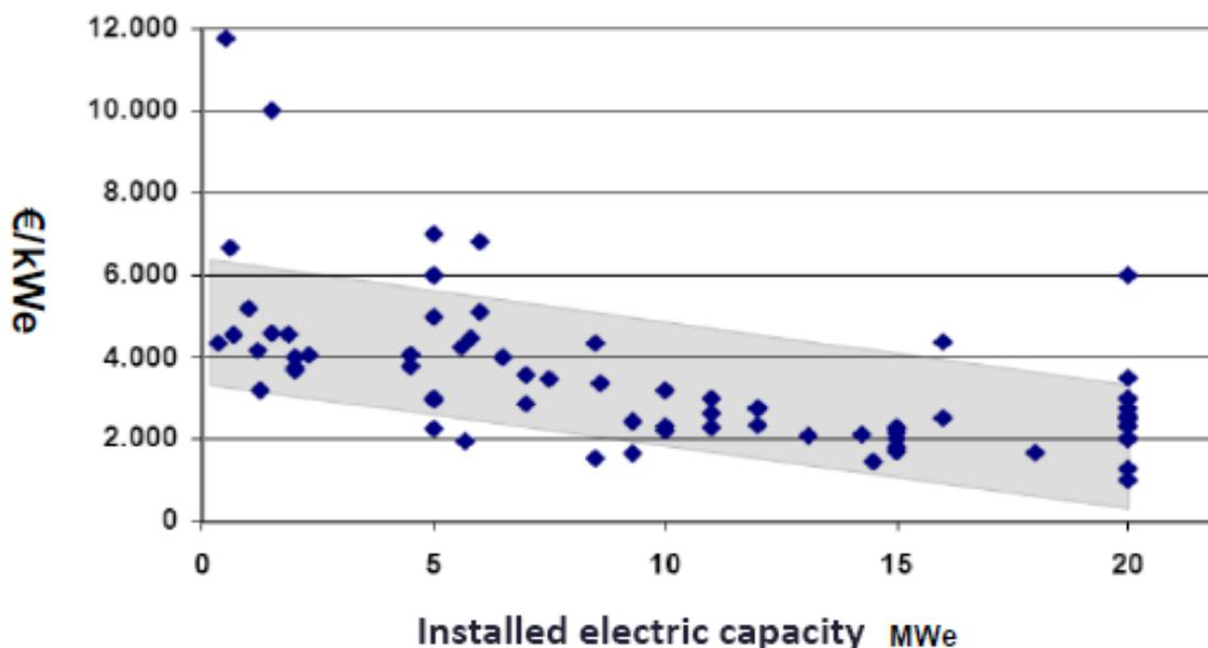
Figure 3.7 Specific investment cost of cogeneration plant for district heating
