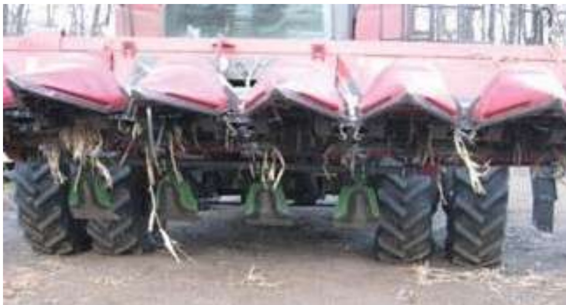
Fig. 20 Corn header with Stalk Stompers
