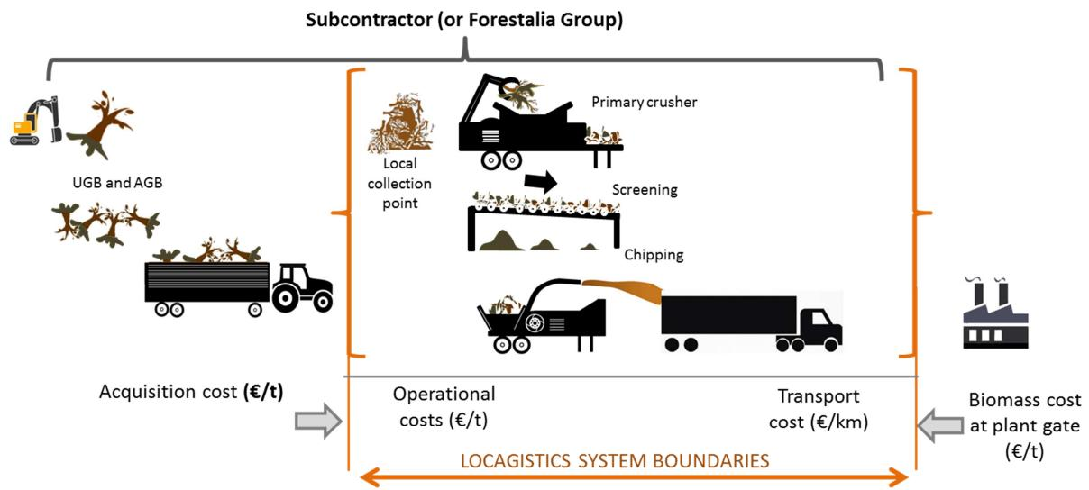
**Figure 7. Case 2.2: supply chain for AGB and UGB from small plantations, remove and transport to collection point by Forestalia Group.**
